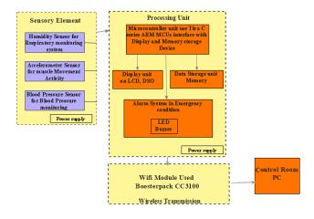
Figure 4. Block diagram
