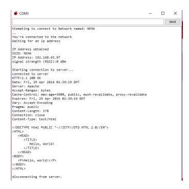
Figure 8. Wi-Fi module connected to the host server
